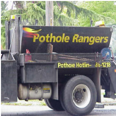
Figure 28: Pothole patching truck with a hotbox
