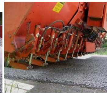
Figure 21. Individual chip gates—this arrangement allows for variable chip application rates.
