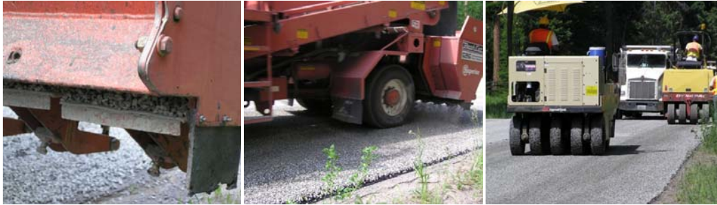
Figure 22. Close-up of chip distribution gates.
